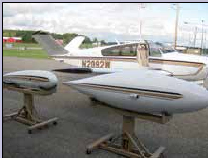
Tip Tanks: 20 gal tips used from 1975-2008; 80 gal Texas Tips used for earthrounding.
