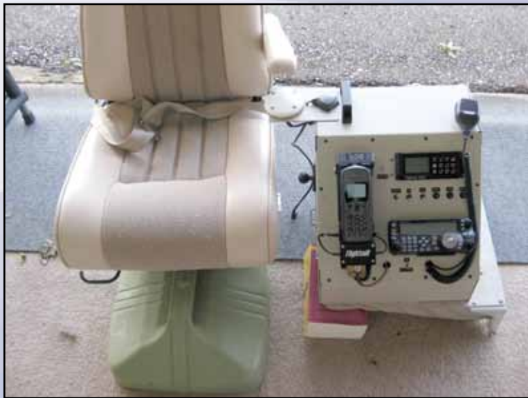
The oceanic cabinet rests on the copilot seat with seatback removed, same bolts mount the cabinet which tilts back for exit and entry. Cabinet contains HF, satellite phone, DZM tracking device and Vistanav synthetic vision backup glass panel.
