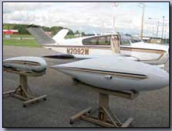
Tip Tanks: 20 gal tips used from 1975-2008; 80 gal Texas Tips used for earthrounding.
